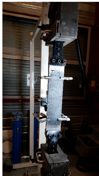
Figure 2. Tensile test setup.
