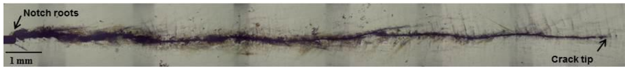
Figure 4 - Nearly-transverse secondary branches in mode II for 16NCD13 steel
