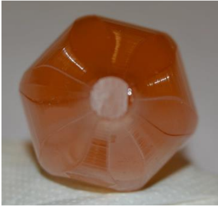
Figure 6. Facets of LGT crystal ( \phi \approx 50 mm) grown under stationary stable regime along Z-axis
