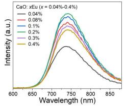
**Figure S13.** PL spectra of CaO:xEu (x = 0.04%-0.4%) under 470 nm excitation.
