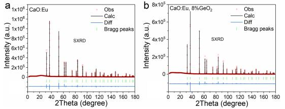
**Figure S10** a-b) Rietveld refinement of the synchrotron XRD profile for CaO:Eu and CaO:Eu, 8%GeO<sub>2</sub>.
