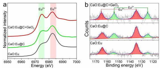
**Figure S3** a) XANES spectra of the Eu L3 edge for CaO:Eu, CaO:Eu@C and CaO:Eu@C+GeO<sub>2</sub> samples. b) XPS spectra of Eu3*d* region recorded for CaO:Eu, CaO:Eu@C and CaO:Eu@C+GeO<sub>2</sub> samples.
