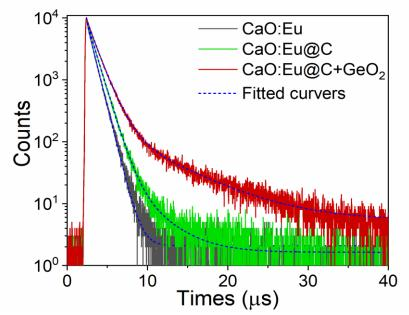
**Figure S4** Photoluminescence decay curves of the different phosphors under 450 nm pulse laser diode excitation. The statistical photons are 10000. All the datas were fitted by the FAST software attached with FL1000.
