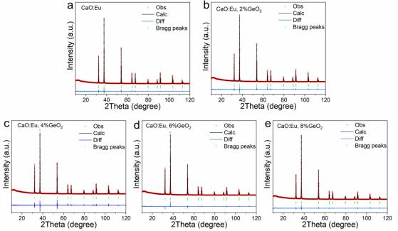
**Figure S9** a-e) Rietveld refinements of CaO:Eu, xGeO<sub>2</sub> samples: x = 0.8% based on XRD datas.
