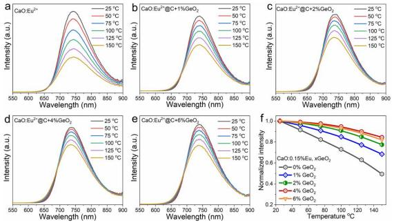
**Figure S5** a-e) Temperature-dependent emission spectra of CaO:Eu@C+xGeO<sub>2</sub> (x = 0.6%) phosphor under 470 nm excitation in the temperature range 25-150 °C with a temperature interval of 25 °C. f) Temperature dependence of the relative integrated photoluminescence intensity for CaO:Eu@C+xGeO<sub>2</sub>.
