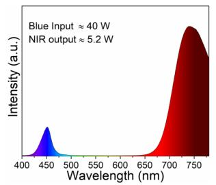
**Figure S12** PL spectra of the fabricated high-power NIR-LED based on four InGaN chips (460 nm, 10 W) and CaO:Eu@C+4%GeO<sub>2</sub> phosphor.
