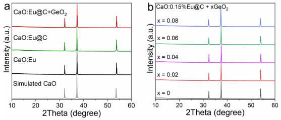
**Figure S1** Structural characterization of CaO:Eu phosphor. a) X-ray powder diffraction patterns of CaO:Eu, CaO:Eu@C, CaO:Eu@C+GeO<sub>2</sub> and the calculated pattern based on Rietveld refinement data (gray line). b) XRD patterns of CaO:Eu, xGeO<sub>2</sub> (x = 0.8%) samples.
