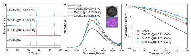
**Figure S11** a) XRD patterns of CaO:Eu@C+xSnO<sub>2</sub> (x = 0-1.5%) phosphor. b) PL spectra of CaO:Eu@C+xSnO<sub>2</sub> under 470 nm excitation, and the photographs of crucible lid and CaO:Eu@C+SnO<sub>2</sub> phosphor. c) Temperature-dependent emission spectra of CaO:Eu@C+xSnO<sub>2</sub> phosphor in the temperature range 25-150 °C. Note: Similar Sn particles observed on the crucible lid suggests that Sn do not enter CaO host lattice.
