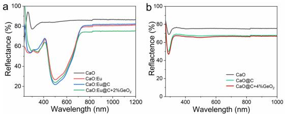
Figure S2 a) UV-vis diffuse reflectance spectra of CaO, CaO:Eu, CaO:Eu@C and CaO:Eu@C+4%GeO<sub>2</sub>. powder. b) UV-vis diffuse reflectance spectra of CaO, CaO@C and CaO@C+GeO<sub>2</sub> host.
