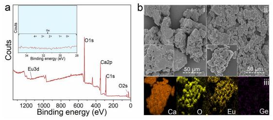
**Figure S8** a) XPS spectra of CaO:Eu, 4%GeO<sub>2</sub>. b) SEM images of CaO:Eu@C (i) and CaO:Eu@C+4%GeO<sub>2</sub> (ii) particles; and (iii) the element mapping images of Ca, O, Eu, and Ge for the selected particle.
