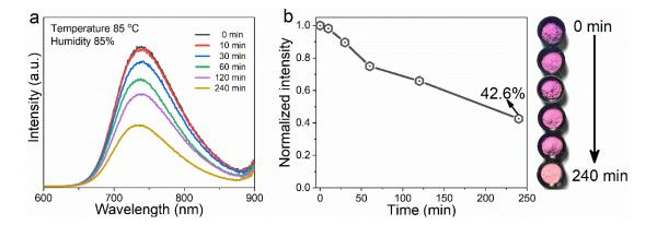
Figure S14. a) The PL spectra of the pristine CaO:Eu and samples treated in degradation conditions at 85% relative humidity (RH), 85  $^{\circ}$ C for different time, respectively. b) The normalized integrate PL intensities dependent on times and photographs of these samples under natural light.
