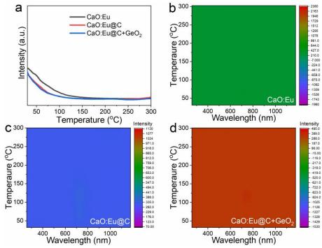
**Figure S6** a) Thermoluminescence curves of CaO:Eu, CaO:Eu@C and CaO:Eu@C+4%GeO<sub>2</sub> in the temperature range 25-300 °C. b-d) 3D- thermoluminescence spectra of CaO:Eu, CaO:Eu@C and CaO:Eu@C+4%GeO<sub>2</sub> after 254, 395 and 450 nm irradiation for 100 s at room temperature.
