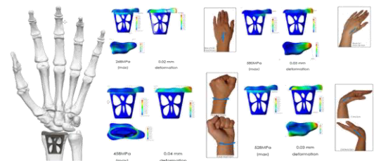
Figure 13: FEM simulation of a new patient-specific prosthesis for resurfacing of the distal radius based on different scenarios (CAE tool: Solidworks® ), Courtesy of [36]
