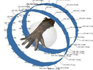
Figure 3: 3D hand reconstruction using photogrammetry (blue planes are identified camera image planes), courtesy of [9]
