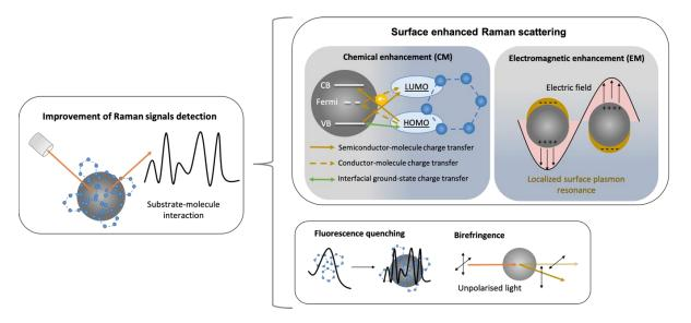
**Figure 2.** Illustration of Raman signal enhancement mechanisms, based on (EM) electromagnetic field interacting with a metal sphere; (CM) electron transfer between a particle and a molecular adsorbate (yellow and green arrows); (Fluorescence quenching) illustration of the quenching of fluorescence process: formation of an adsorbate/metal complex resulting in an additional channel of nonradiative return to ground state; (birefringence) in chiral substrates.
