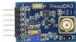
FIGURE 5 – DAC PmodDA3 board.
