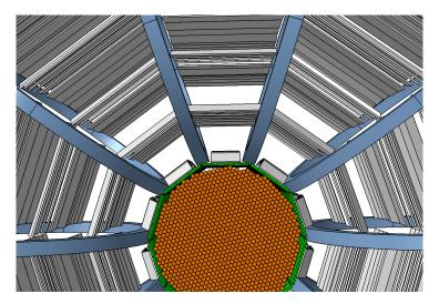
**Figure 13.** Detailed rendering of the front view of the ALADInO calorimeter (orange) placed in the center of the apparatus.
