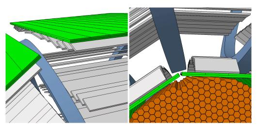
**Figure 15.** Details of the baseline layout proposed for the ToF outer (**left**) and inner (**right**) rings. The ToF plastic scintillating counters are shown in green, together with the magnet coils (blue), the silicon tracker sensors (gray), and the calorimeter crystals (orange).
