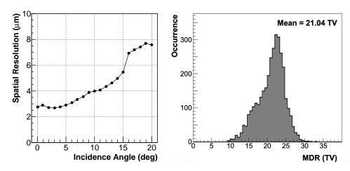
**Figure 10.** Left: Spatial resolution of the PAMELA tracker short ladders as a function of the particle incident angle. Figure recreated by authors of [142] from original data files, see original paper for details. Right: Distribution of the MDR of the ALADInO spectrometer evaluated with preliminary numerical simulations over a wide range of incident angles. The result confirms the reach of an average MDR larger than 20 TV for the expected tracker coordinate resolution.
