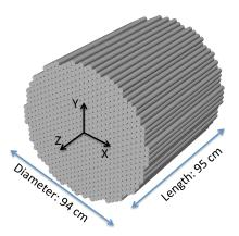
**Figure 11.** Representation of the active volume of the ALADInO calorimeter. 15925 LYSO crystals are arranged in a total assembly of 637 lines, each made of 25 aligned hexagonal prism crystals. Figure readapted from [96] under license CC BY 4.0.
