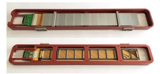
**Figure 8.** Picture of an AMS-02 ladder made of 12 double-sided  $40 \times 70 \,\mathrm{mm}^2$  silicon microstrip sensors, enclosed in a plastic transport box. Strips measuring the bending direction are readout using a daisy-chain microbonding connection (top view), while transversal strips are readout via additional routing provided by a metalized Upilex film (bottom view), such that the FEE readout is located at the longitudinal edge of the ladder.
