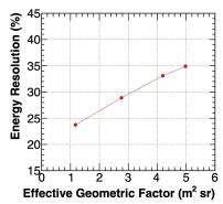
**Figure 14.** Left: distribution of the shower length in the calorimeter after the point of first hadronic interaction for 1 TeV protons impinging isotropically on the calorimeter. Right: dependence of the energy resolution for 1 TeV protons as a function of the effective geometric factor defined by a selection on the calorimeter fiducial volume and on the particle pathlength inside the calorimeter crystals.
