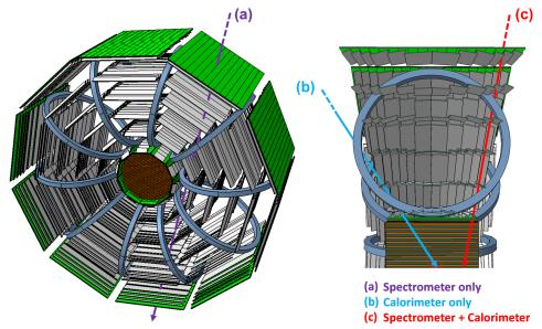
**Figure 3.** Graphical illustration of the main acceptance configurations of the ALADInO detector for high-energy particles (straight tracks). (a) Particle crossing the spectrometer only; (b) particle crossing the calorimeter only; (c) particle crossing the spectrometer and the calorimeter. Figure readapted from [96] under license CC BY 4.0.
