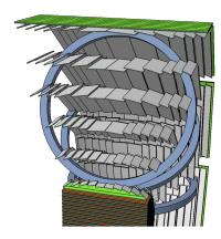
**Figure 9.** Detailed rendering of the silicon ladder orientation in the ALADInO tracker, optimized to reduce the occurrence of particles with large incident angles in the tracker sensor acceptance. Figure readapted from [96] under license CC BY 4.0.
