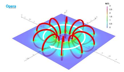
**Figure 7.** Schematic rendering of the magnet and map of the generated magnetic field in the configuration of 10 round coils with the geometry discussed in the text. The field has been simulated using [126]. The white arrow sketches the direction of the magnetic field inside the coils. Figure readapted from [96] under license CC BY 4.0.
