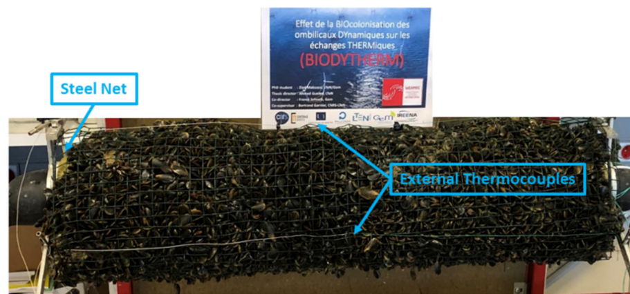
Figure 6. Uniform distribution of mussels around the experimental tube held by a steel net.
