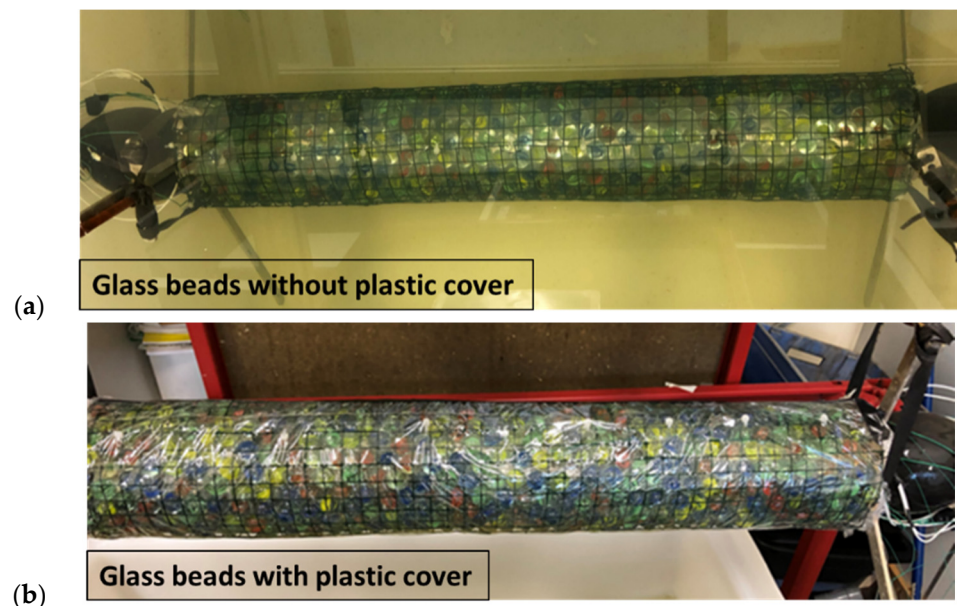
Figure 9. Experimental tube covered with glass beads (a) without plastic cover (b) with plastic cover.
