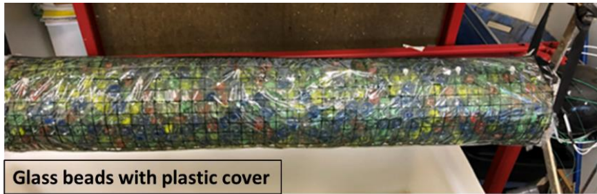
Figure 9. Experimental tube covered with glass beads (a) without plastic cover (b) with plastic cover.
