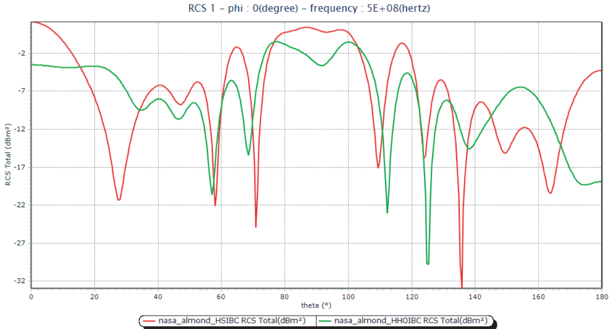
Figure 5: \phi\phi component of the monostatic RCS for a coated conducting almond, PMCHWT solution, SIBC solution and HOIBC solution.
