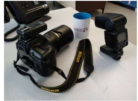
(d) Equipment for the 3D scan: a DSLR and a flash connected via a wireless radio command.
