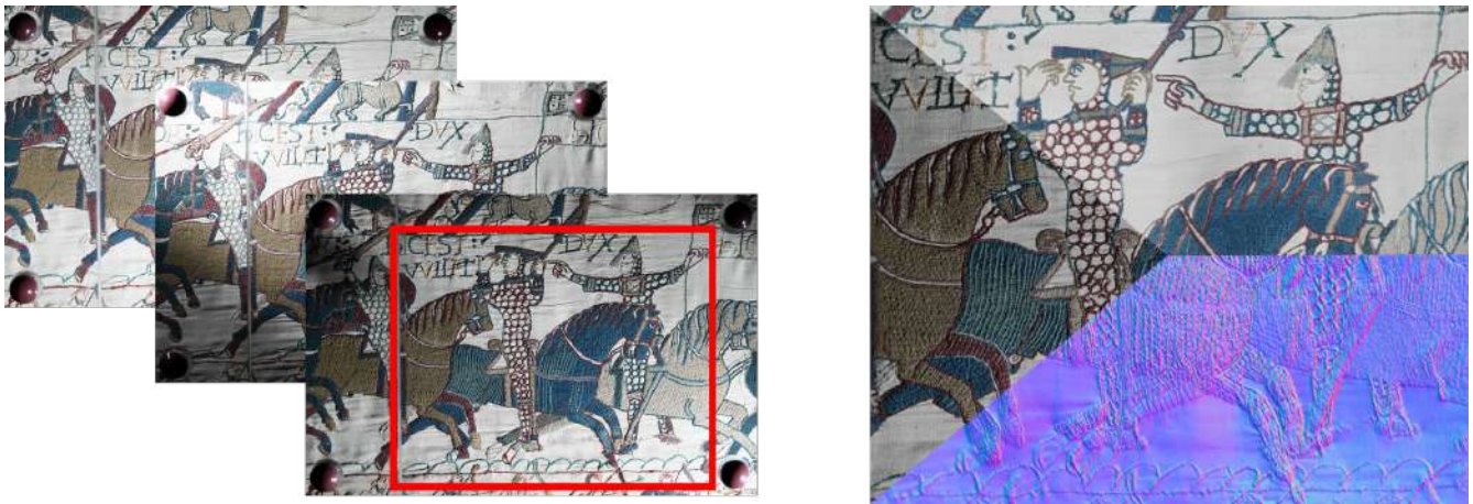
Figure 10. Left: 3 (out of 12) images of William revealing his face (scene 55). Right: using photometric stereo in the area highlighted in red, the input image sequence (one image of the sequence is recalled on the left) can be decomposed between reflectance (top, right) and normals (shown in false colors on bottom, right). Reflectance encodes the scene's color, independently from shape and illumination: see how the folds on the linen canvas have been eliminated. Normals, on the other hand, encode the scene's micro-geometry through the surface's orientation, which reveals thin details such as wool strings.
