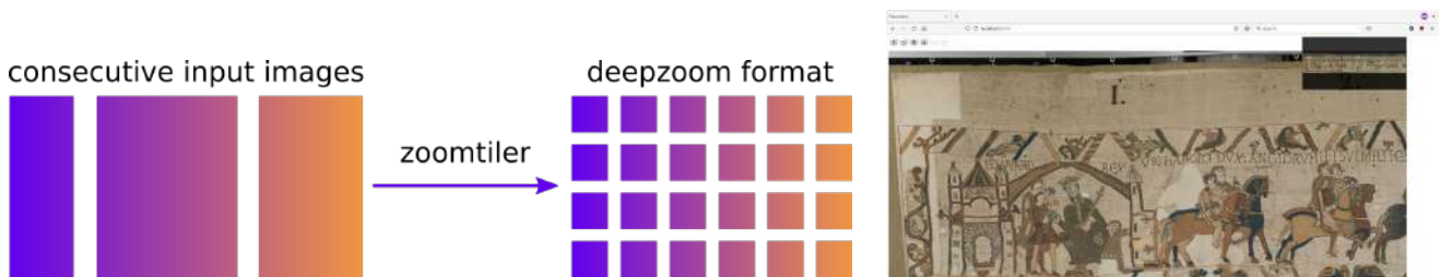
Figure 5. Left: Zoomtiler, a simple CLI program to generate zoomable tiled images from a horizontal succession of images. Right: OpenSeadragon Web image viewer used on a small section of the Bayeux Tapestry. Users may navigate through the entire content of the embroidery with their mouse, and also easily switch between the different imaging modalities, as illustrated in Figure 2.
