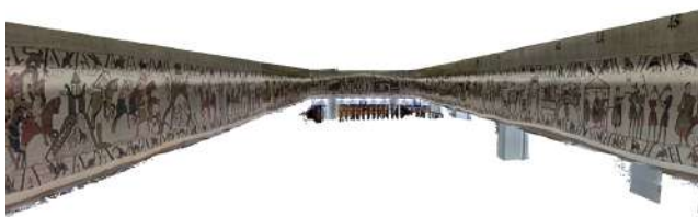
(a) Dense point cloud representing the whole photogrammetric 3D-reconstruction.
