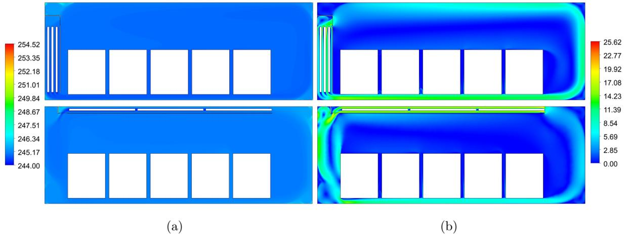
Figure 11: (a) Temperature [K] and (b) velocity magnitude [ms<sup>-1</sup>] contours of Configuration A with cargo (top) and Configuration B with cargo (bottom).
