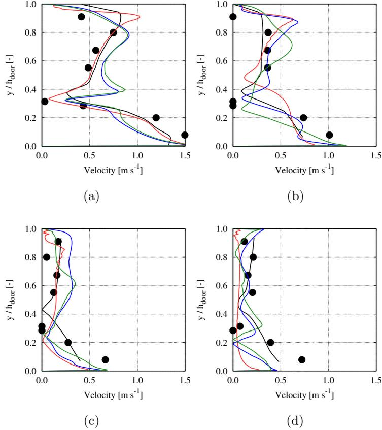
Figure 4: Comparison of the velocity magnitude profiles at the container door vertical centerline between the present simulations and the published data of Lafaye de Micheaux *et al.* [1] at (a)  $t = 10$  s, (b) 20 s, (c) 40 s and (d) 60 s. Legend: • Experiment - Lafaye de Micheaux *et al.* [1], — CFD - Lafaye de Micheaux *et al.* [1], — CFD 3D, — CFD 2D with no heat transfer, — CFD 2D with heat transfer.
