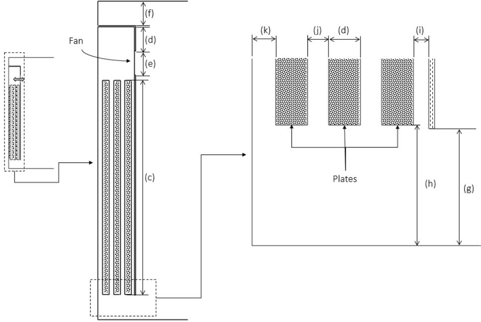
Figure 2: Details and dimensions of the eutectic plates.
