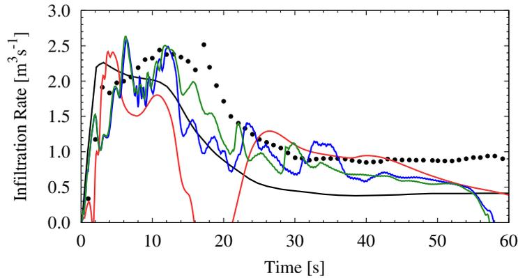
Figure 6: Comparison in terms of the infiltration rate at the container door between the present simulations and the experimental
