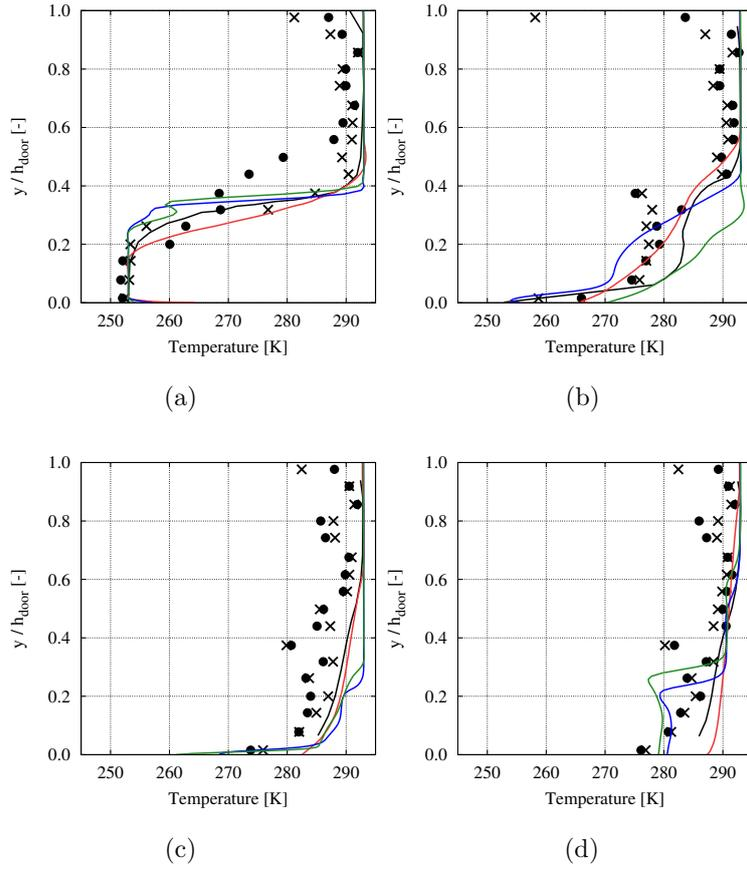
Figure 5: Comparison of the temperature profiles at the container door vertical centerline between the present simulations and the published data of Lafaye de Micheaux *et al.* [1] at (a)  $t = 10$  s, (b) 20 s, (c) 40 s and (d) 60 s. Legend: • Experiment 1 - Lafaye de Micheaux *et al.* [1], × Experiment 2 - Lafaye de Micheaux *et al.* [1], — CFD - Lafaye de Micheaux *et al.* [1], — CFD 3D, — CFD 2D with no heat transfer, — CFD 2D with heat transfer.
