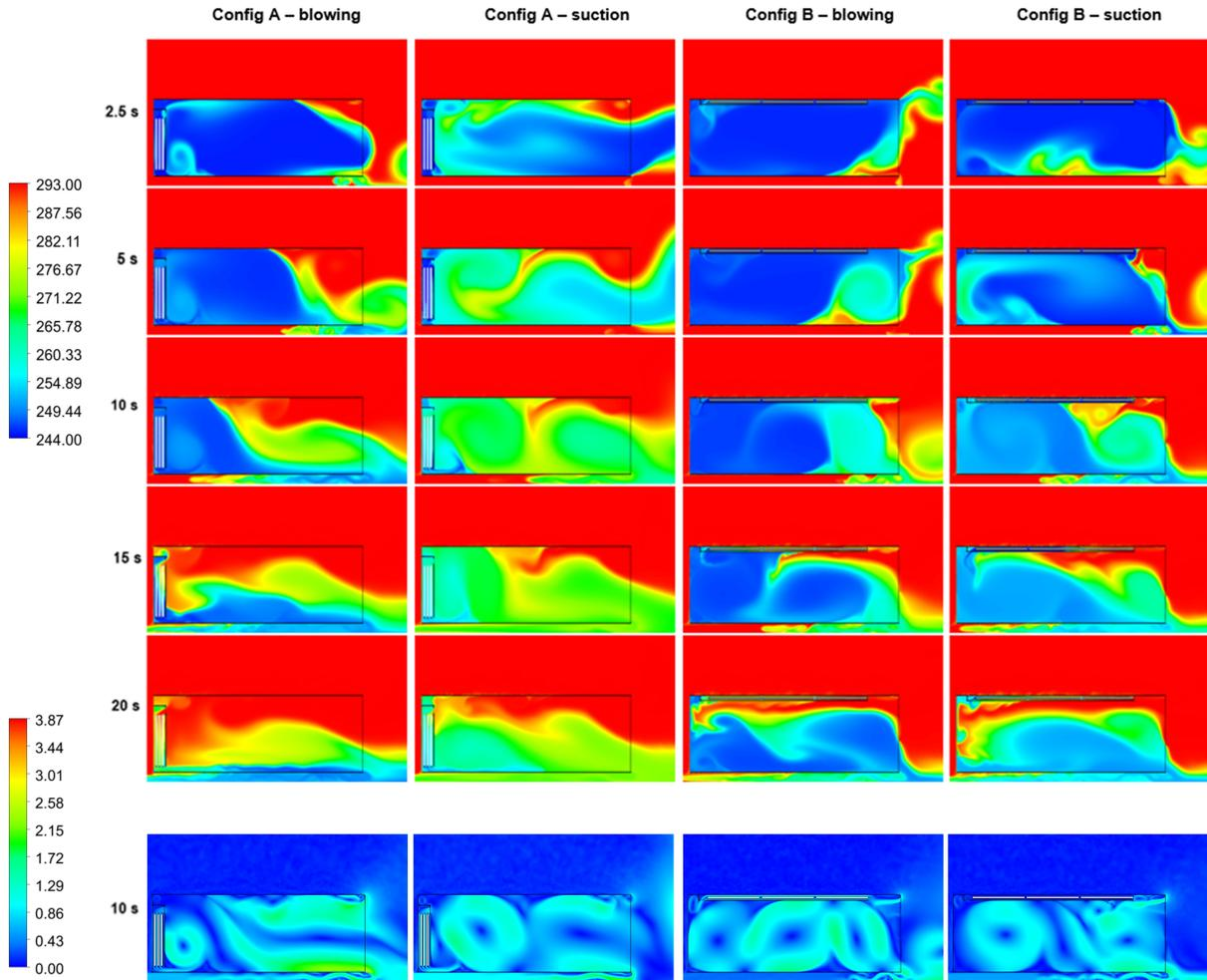
Figure 10: (top) Time evolution of the temperature contours [K] for both configurations and fan modes at five instants; (bottom) Corresponding velocity magnitude contours [ms<sup>-1</sup>] at  $t = 10$  s.
