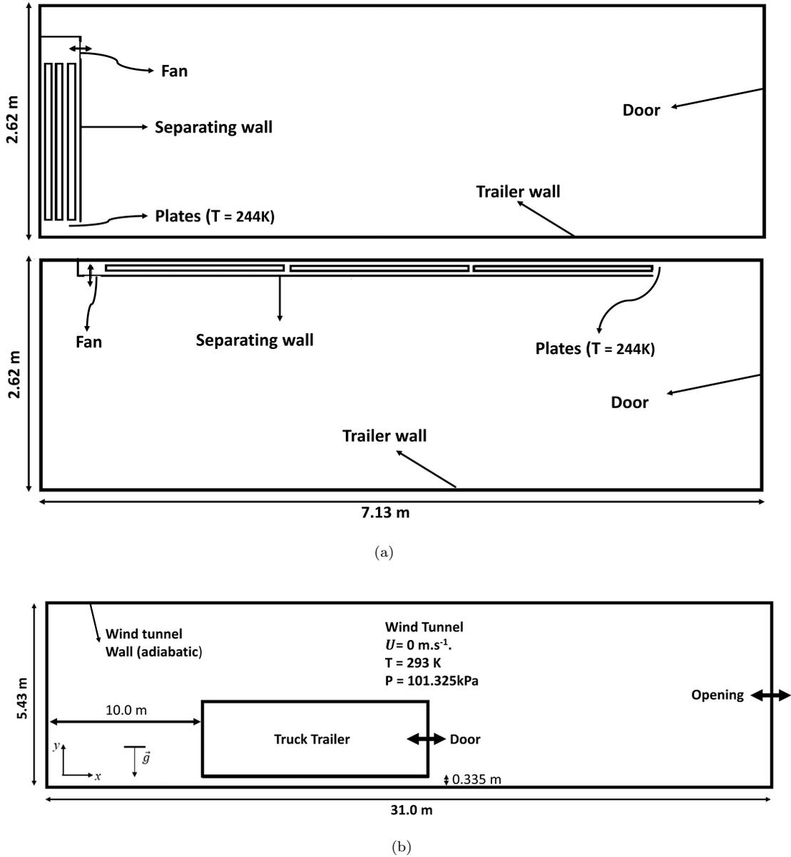
Figure 1: (a) Trailer diagram with the position of the eutectic plates for Configuration A (top) and Configuration B (bottom)
