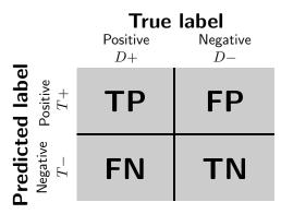
**Figure 1**: Confusion matrix The confusion matrix represents the results of a classification task. In the case of binary classification (two classes), it divides the test samples into four categories, depending on their true (eg disease status, D) and predicted (test output, T) labels: true positives (TP), true negatives (TN), false positives (FP), false negatives (FN).
