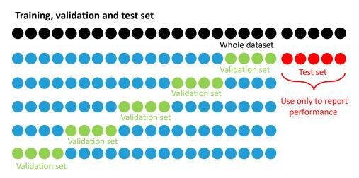
Use to train the model, experiment with different architectures...
