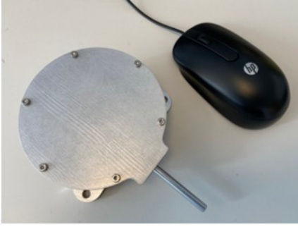
Fig. 2: Picture of the packaging of the 8cm-diameter PBG-HCF ring resonator (computer mouse for scale)
