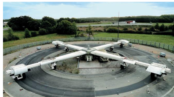
Figure 3 : Fatigue carousel at the Gustave Eiffel University (Nantes)
