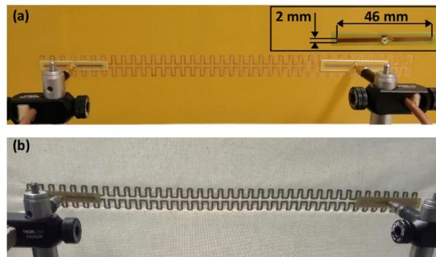
**Fig. 4.** Experimental setup for determining the odd mode transmission of the meandered TL fabricated by (a) PCB (Kapton) and (b) embroidery technique, respectively. In inset, the geometric sizes of the dipole antenna.
