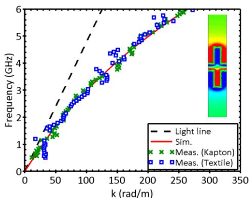
**Fig. 2.** Simulation (Sim.) and measurements (Meas.) of the dispersion curve of the odd mode supported by the meandered TL. In inset,  $z$ -component of the magnetic field ( $H_z$ ).
