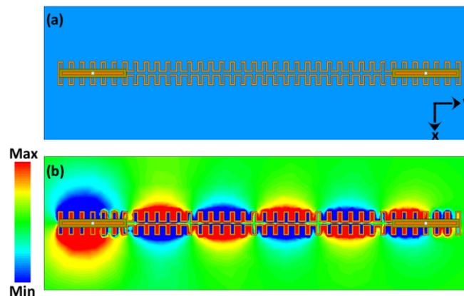
**Fig. 3.** (a) Simulated meandered TL and the wirelessly excited odd mode propagation by means of dipole antennas in horizontal polarization. (b)  $z$ -component of the magnetic field ( $H_z$ ) plotted in the  $x$ - $y$  plane at  $f = 2.15$  GHz.
