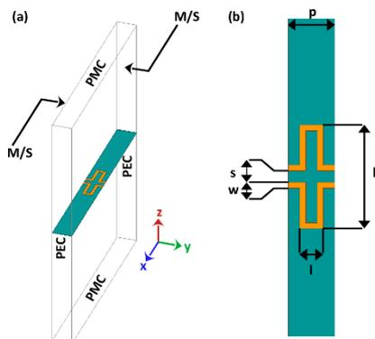
**Fig. 1.** Unit cell of the meandered TL used to calculate the dispersion curve with (a) boundary conditions and (b) geometric sizes with  $p=8$  mm,  $h=18$  mm,  $s=2$  mm,  $w=1$  mm and  $l=4$  mm.
