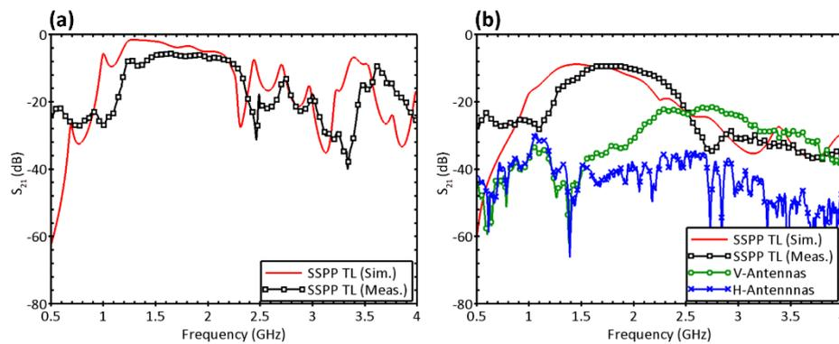
**Fig. 5.** Simulated (Sim.) and measured (Meas.) transmission for the odd mode supported by the (a) PCB and (b) embroidered SSPP TL. (b) Comparison with the transmission measured in free space between vertical-oriented (V-Antennas) and horizontal-oriented (H-Antennas) antennas.
