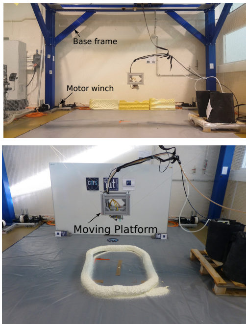
Figure 4. A CDPR, named CRAFT, used for foam additive manufacturing at LS2N, Nantes, France
