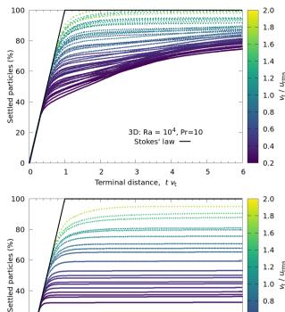
**Figure 9:** The percentage of settled particles as a function of time. Each line represents one of the 201 particle types, only those with  $0.2 < |v_{\rm t}|/u_{\rm rms} < 2.0$  are shown. The x-axis represents the terminal distance,  $t\,v_{\rm t}$ , solid black line is the Stokes' law, i.e. the solution for sinking in a quiescent fluid.
