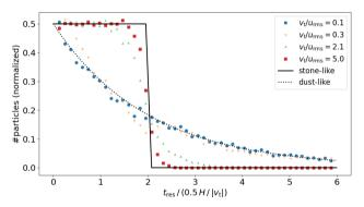
**Figure 2:** Probability density function of  $t_{\rm res}$  for  $Ra=10^6$  and Pr=1. The analytical distributions for the dust-like (dotted black line) and stone-like (solid black line) regimes stem from Eq. (8), upon considering the concentration at the settling front to be either N(t)/H (dust-like regime) or  $N_0/H$  (stone-like regime).
