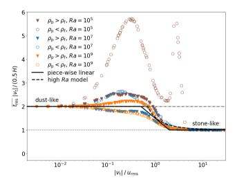
**Figure 11:** Same as Fig. 1, only here for internally instead of basally heated convection. Because of flow asymmetry, the residence times are different for the light and for the heavy particle types (empty circles vs. filled triangles). As Ra increases,  $\overline{t_{res}}$  approaches the high-Ra model from Eq. (13).
