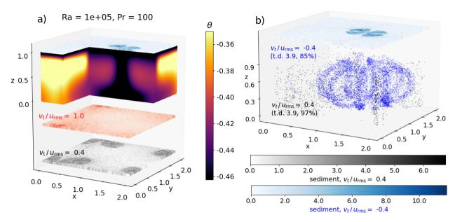
**Figure 10:** Same as panels a) and b) in Fig. 3, only here the convection is internally driven, with the equivalent Rayleigh number being  $10^5$ , and for a higher Prandtl number Pr=100. This time we show also the distribution of light particles with  $v_{\rm t}/u_{\rm rms}=-0.4$  (blue dots). These particles are focused in a two spherical clouds centred at conduits of the two dominant downwellings, and are deposited preferentially at their roots.
