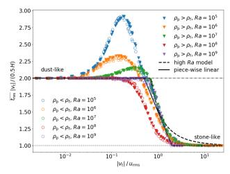
Figure 1: Mean residence time of the particles, normalized by the mean terminal time  $0.5\,H/|v_{\rm t}|$ . Triangles represent heavy particles, i.e. the particle types with  $\rho_{\rm p}/\rho_{\rm f} \in (1-2]$ , while open circles stand for light particles,  $\rho_{\rm p}/\rho_{\rm f} \in [0-1)$ . Black line represents the high-Ra model towards which the results converge when Ra is increased.
