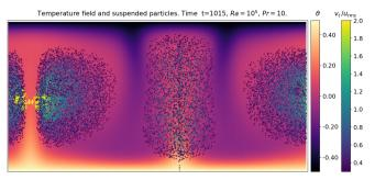
**Figure 8:** Particles that are still suspended at the time  $t \approx 1000$  in 2D basally heated convection with  $Ra = 10^5$ , Pr = 10. Only the particle types satisfying  $0.3 < v_1/u_{\rm rms} < 3.0$  are plotted.
