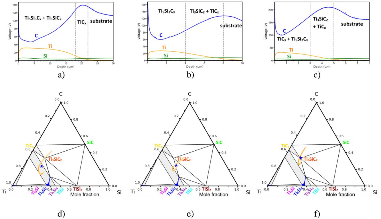
Figures 11. GDOES profiles measured on SiC monoliths heated at  $1200^\circ\text{C}$  for 2h: emission profile: a) without Si addition; b) with addition of 0.5g of Si; and c) with addition of 1g of Si; and atomic quantification: d) without Si addition; e) with addition of 0.5g of Si; and f) with addition of 1g of Si. The mean compositions are localized by blue five-pointed stars.
