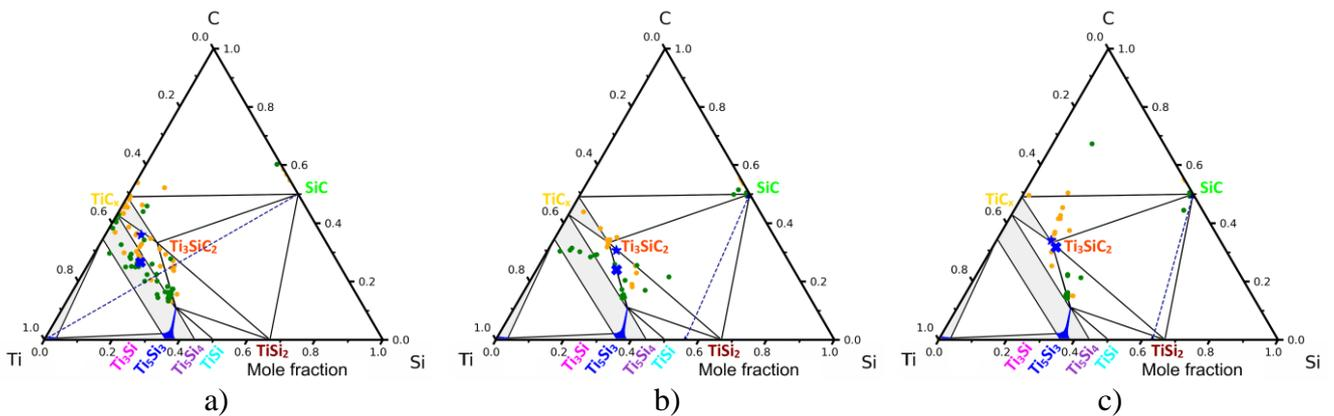
Figures 10. Localization in the Ti-Si-C phase diagram of the EDS (orange points) and WDS (green points) measurements on  $\text{SiC}$  monoliths heated at  $1200^\circ\text{C}$  for 2h: a) without Si addition; b) with addition of 0.5g of Si; and c) with addition of 1g of Si. The mean compositions are localized by blue five-pointed stars (EDS) and blue saint Andrew's crosses (WDS).
