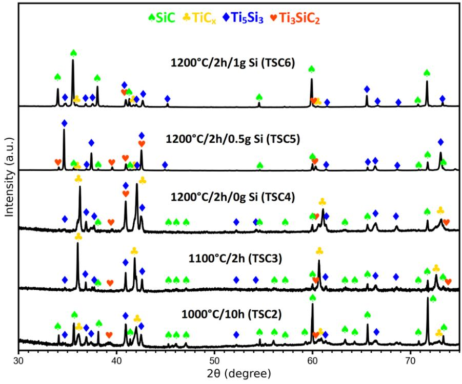
Figure 5. XRD patterns of the coatings and remaining powders from molten salts synthesis at 1000°C, 1100°C, and 1200°C.
