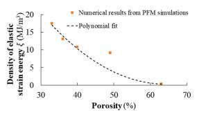
Fig. 16. Evolution of the density of elastic strain energy as a function of porosity ( $\ell=0.8~\mu m).$
