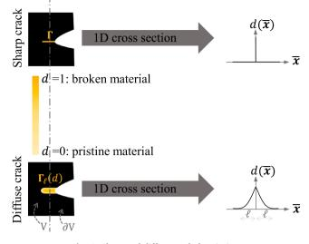
Fig. 6. Sharp and diffuse crack description.
