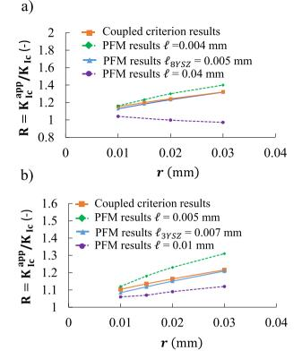
**Fig. 10.** The dependence of the relative toughness on the cavity radius considering different values of the length scale parameter  $\checkmark$  for: a) 8YSZ material, b) 3YSZ material.  $\measuredangle_{8YSZ}$  and  $\measuredangle_{3YSZ}$  refer to the length scale parameters that provide close agreement between the coupled criterion and the PFM results over the whole considered range of cavity radii.
