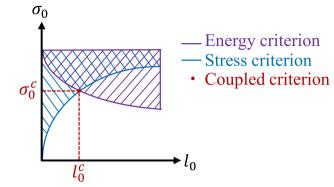
**Fig. 5.** Applied loading as a function of the initial crack length for the coupled criterion obtained using the stress (in blue) and the energy (in purple) criteria. The coupled criterion is chosen among the admissible solutions such  $l_0^c$  minimizes the applied loading  $\sigma_0^c$  (in red). (For interpretation of the references to colour in this figure legend, the reader is referred to the web version of this article.)
