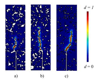
Fig. 11. Cartographies displaying the crack path within the porous microstructures: a) first realization at  $\varepsilon = 20$  %, b) second realization at  $\varepsilon = 20$  %, c) first realization at  $\varepsilon = 10$  %. ( $\ell_{3YSZ} = 0.1 \ \mu m$ ).
