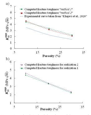
**Fig. 13.** Experimental and simulated dependences of the apparent fracture toughness on porosity using a) the two computation methods for realization 1, b) "method 1" for the two realizations.
