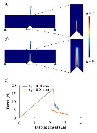
**Fig. 7.** Visualization of the crack pattern initiated from a notch at an opening angle  $2\beta$  of 90° for: a)  $\ell_1 = 0.01$  mm, b)  $\ell_2 = 0.04$  mm. c) Force-Displacement curves considering the 8YSZ material at a V-notch angle  $2\beta$  of 90° for $\ell_1 = 0.01$  mm and  $\ell_2 = 0.04$  mm.
