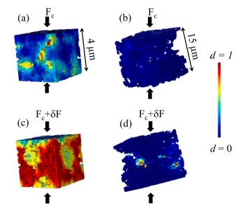
**Fig. 15.** Visualization of the cracks created in porous microstructures submitted to compression: First micro-cracks created in the microstructure for a porosity of a) 33 % and b) 63 %. Evolution of the damage variable after a small increment of charge at c) 33 % and d) 63 % ( $\ell = 0.4 \mu m$ ).
