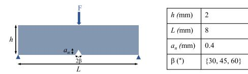
Fig. 1. Three-point-bending test on a V-notched sample.
