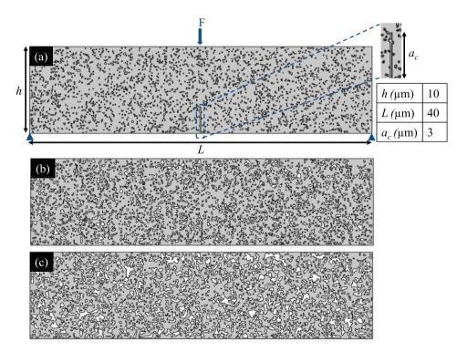
Fig. 3. Synthetic porous microstructures at different porosity volume fractions ε (solid phase in grey): a) 10 %, b) 20 %, c) 30 %.
