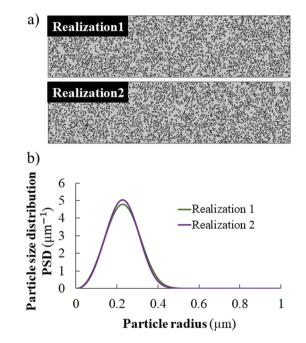
Fig. 12. Comparison between two generated synthetic microstructures with  $\varepsilon$  = 20 %: a) visualization of the two realizations of the microstructure, b) Solid phase size distributions computed on the two realizations.
