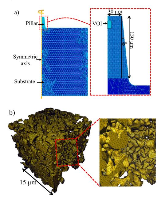
Fig. 4. Mesh of the: a) tapered pillar attached to the pellet with axisymmetric conditions. A zoom on the pillar is shown together with the location of the Volume Of Interest (VOI) for the simulation at the microstructure scale, b) 3D microstructure at a porosity of 63 %.
