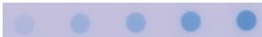
Figure 1. Scan of OC-1 film irradiated at 2,5,10,20 and 30Gy, respectively from left to right.
