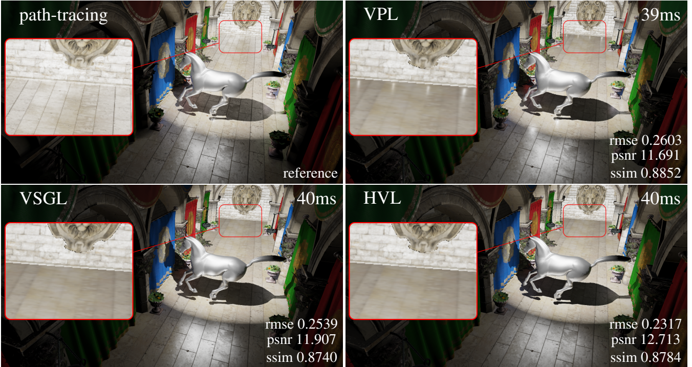
Figure 12: Comparison with 900 VPL, 529 VSGL and 400 HVL, generated at equal time. Images are rendered at 1600 \times 900 . The HVL cache resolution is 322^2 pixels, and 14^2 pixels for one VSGL. The contribution of HVLS is on 15 SH bands. In this rendering, HVL are limited to circularly symmetric specular lobe to compute lighting only on ZH. Insets show VPL spike artifacts and VSGL or HVL robustness to those artifacts. See additional material for more comparisons and implementation details.
