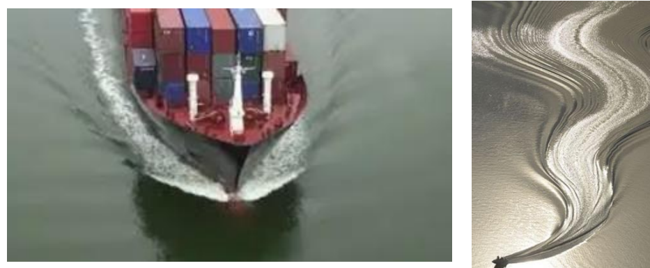
Figure 7. Bow waves alongside and in front of boat and standing wave behind fast-moving boat on the right.
