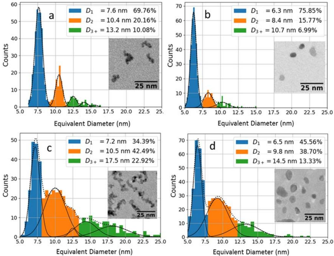
**Fig. 1.** Size histograms with N-Gaussian fit (black curves), separation of NPs population in monomers  $D_1$  (in blue), dimers  $D_2$  (in orange) and the rest for larger diameters as  $D_{3+}$  (in green) with corresponding % of NPs and TEM image in insert, for LD as prepared (a), LD annealed (b), HD as prepared (c) and HD annealed (d) large FeRh samples.
