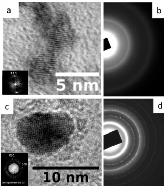
**Fig. 2.** High resolution TEM images of nanoparticles, with corresponding Fast Fourier Transform in insert (a and c) and electron diffraction pattern (b and d) before and after annealing, respectively.
