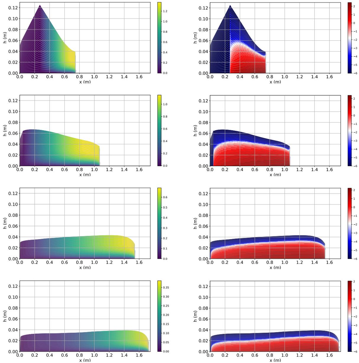
Figure 9: Velocity field (left-hand side), and  $\log_{10}(|\partial_z u|)$  (right-hand side) for  $\theta = 15^\circ$  at times  $t = 0.2, 0.5, 1.0, 1.5$  s during the inertial phase of the flow, computed with model (10). We use 32 vertical layers here.
