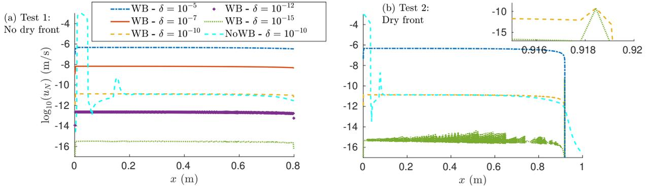
Figure 4: Maximum velocity ( $\log_{10}(u_N)$ ) for the considered steady state tests for different values of the regularization parameter ( $\delta$ ) at  $t = 10$  s, and also the well-balanced discretization in (26). Inset figure in (b) Test 2 is a zoom of the front position.
