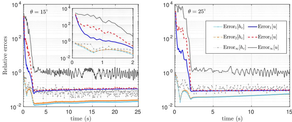
Figure 12: Relative differences in semilog scale between the computed velocity field and interface ( $h_c$ ) between the sheared and unshered layers, and the approximations given by the analytical expressions (30d),(30e) and (31) ( $\partial_x h$  computed with the multilayer height). Left: slope  $\theta = 15^\circ$ . Right: slope  $\theta = 25^\circ$ . We use 32 vertical layers here.
