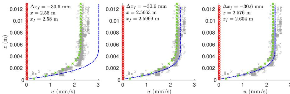
Figure 13: Vertical profiles of velocity at  $x = x_f + \Delta x_f$  for  $\theta = 15^\circ$ . Blue dash-dotted lines are the multilayer results (model (10)), red circles (resp. green crosses) are the analytical profiles (31) with the gradient  $\partial_x h$  computed from the multilayer (resp. experimental) height profile, and gray circles are experimental data of [4]. We use 32 vertical layers here.
