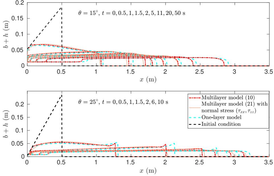
Figure 5: Time evolution of the local free surface, for  $\theta = 15^\circ$  and  $25^\circ$  at different times, with the multilayer model (10) (red dash-dotted lines) and model (21) (orange solid lines), and the one-layer model (cyan dashed lines).
