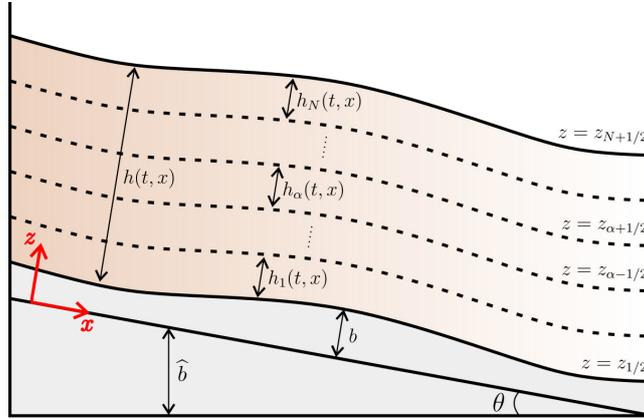
Figure 1: Sketch of the multilayer configuration and notation.
