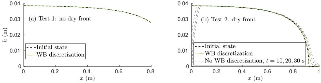
Figure 3: Free surface solutions for (a) Test 1 and (b) Test 2 at the initial time (black dashed line), and at time  $t = 10$  s with the proposed scheme (green dotted lines). Gray dashed lines in (b) are the solutions without the well-balanced treatment in (26). Remind that  $\delta = 10^{-5}$ , here.
