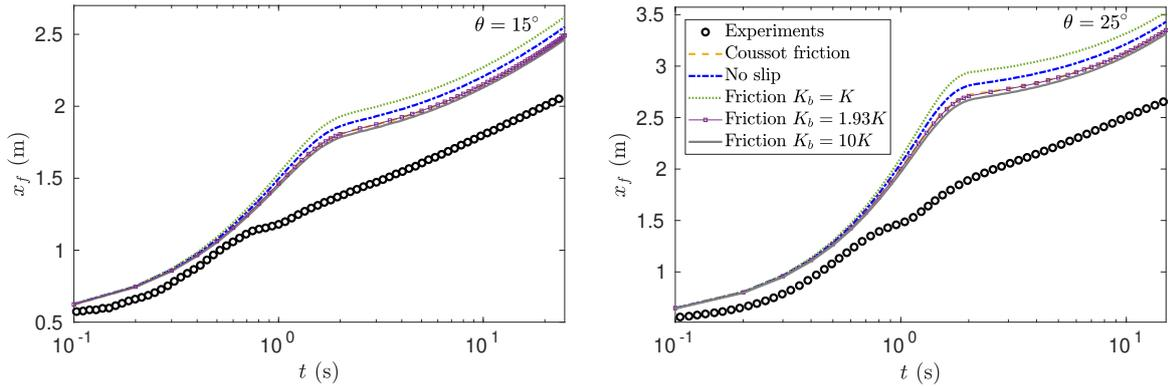
Figure 8: Time evolution of the front position  $x_f$  for  $\theta = 15^\circ$  and  $25^\circ$  with the multilayer model (10) and using different friction conditions: Coussot’s formula (16) (brown dashed lines), no slip (18) (blue dash-dotted lines) and friction condition (15) for several values of  $K_b$  ( $K_b = 1.93K$  corresponds to (17), purple squares). Circles are data experiments.
