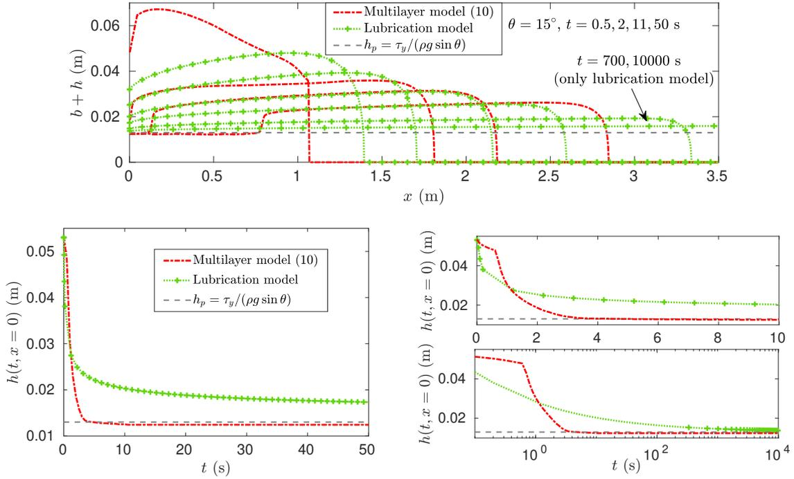
Figure 6: Upper figure: local free surface  $h(x)$  at different times; Lower figures: time evolution of the local free surface at point  $x = 0$  m, for  $\theta = 15^\circ$  with the multilayer model (10) (red dash-dotted lines) and the lubrication model (green (+) lines).
