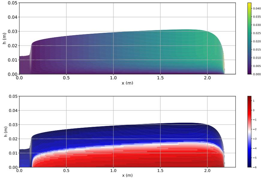
Figure 10: Velocity field (upper figure), and  $\log_{10}(|\partial_z u|)$  (lower figure) for  $\theta = 15^\circ$  at time  $t = 10$  s during the spreading phase of the flow, computed with model (10). We use 32 vertical layers here.
