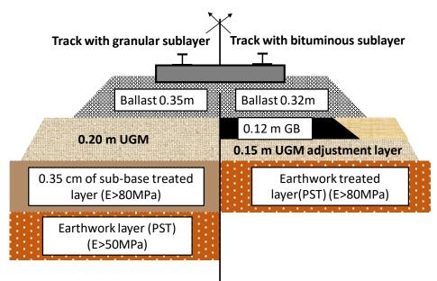
Figure 2. The two experimental structures of the BPL high-speed line (adapted from Khairallah et al., 2019)
