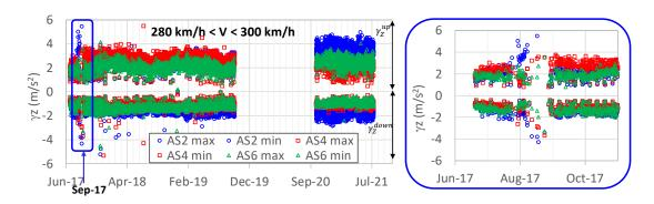
Figure 21. Acceleration under the signal second peak recorded on Section 2 (with granular sub-layer) by accelerometers AS2, AS4 and AS6 at the surface of the UGM layer (located below the outer rail) from July 2017 to July 2021 for 26-bogie trains as a function of time, and zoomed view
