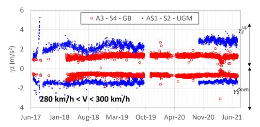
Figure 24. Comparison of positive and negative vertical acceleration peaks, under the signal second peak, recorded on Section 2 (with granular sub-layer) and Section 4 (with bituminous sub-layer) accelerometer AS1 and A3 (both located below the outer rail), respectively, during the commercial phase from July 2017 to July 2021 for 26 bogie-trains and a speed within the range of 280-300 km/h
