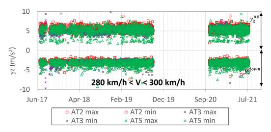
Figure 23. Acceleration under the signal second peak recorded on Section 2 (with granular sub-layer), from accelerometers AT2, AT3 and AT5, located at the top of the sleepers, from July 2017 to July 2021 for 26 bogie-trains and a speed within the range of 280-300 km/h, as a function of time
