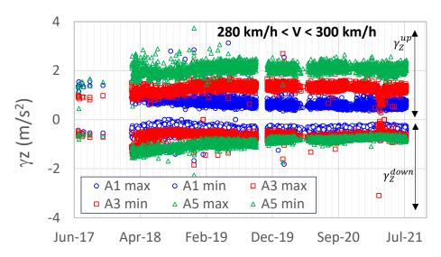
Figure 17. Acceleration under the signal second peak recorded on Section 4 (with bituminous sublayer) by accelerometers A1, A3 and A5 (located under the outer rail) from July 2017 to July 2021 for 26 bogie-trains and a speed within the range of 280-300 km/h as a function of time
