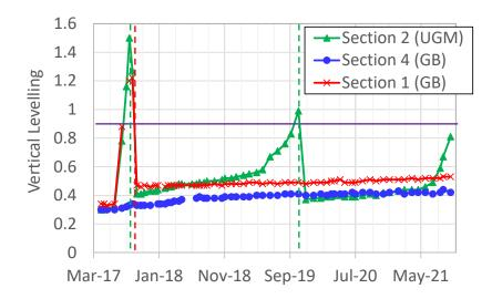
Figure 26. Vertical leveling measured on distances of 200 meters including Sections 2, 1 and 4
