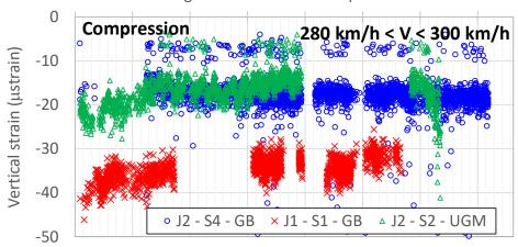
Figure 14. Comparison between the maximum vertical strain values in compression mode measured on Section 2 (with granular sub-layer) and Sections 4 and 1 (with bituminous sub-layer) from July 2017 to July 2021 for 26 bogie-trains and a speed ranging between 280 and 300 km/h
