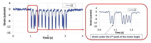
Figure 11. Vertical strain signal (and zooming) recorded on Section 2 (with UGM layer) with J2 strain gauge, V=160 km/h
