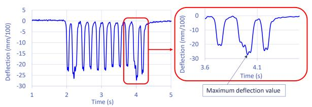
Figure 10. Deflection signal recorded on Section 2 (with UGM layer) with sensor 2, V=320 km/h
