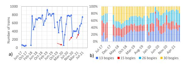
Figure 7. Number on train (a) and distribution of type of train (b) operating, each month, on Section 4 (with bituminous sub-layer)
