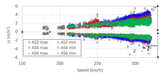
Figure 20. Acceleration under the signal second peak recorded on Section 2 (with granular sub-layer) by accelerometers AS2, AS4 and AS6 at the surface of the UGM layer (located below the outer rail) from July 2017 to July 2021 for 26-bogie trains as a function of speed
