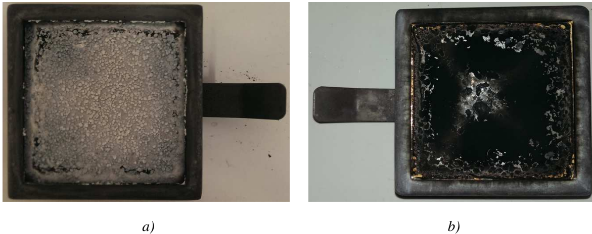
Figure 4: Pictures of the ABS material after testing when the decomposition process is associated with a combustion process a) or flameless b).
