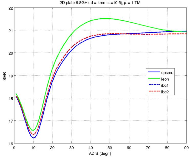
Figure 14: Bistatic RCS for a coated 2D plate, when  $d = 4mm$ ,  $\epsilon_r = 10 - 5j$ ,  $\mu_r = 1.0$ , and  $f = 6.8GHz$  with TM polarization
