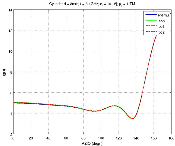
Figure 12: Bistatic RCS for a coated circular cylinder, when  $d = 3mm$ ,  $\epsilon_r = 10 - 5j$ ,  $\mu_r = 1.0$ , and  $f = 3.4GHz$  with TM polarization
