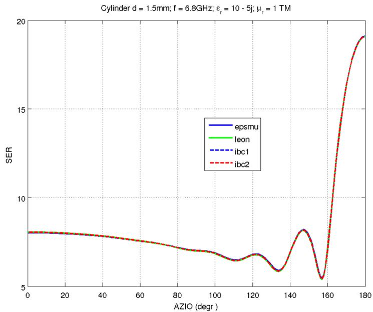
Figure 7: Bistatic RCS for a coated circular cylinder, when  $d = 1.5mm$ ,  $\epsilon_r = 10 - 5j$ ,  $\mu_r = 1.0$ , and  $f = 6.8GHz$  with TM polarization
