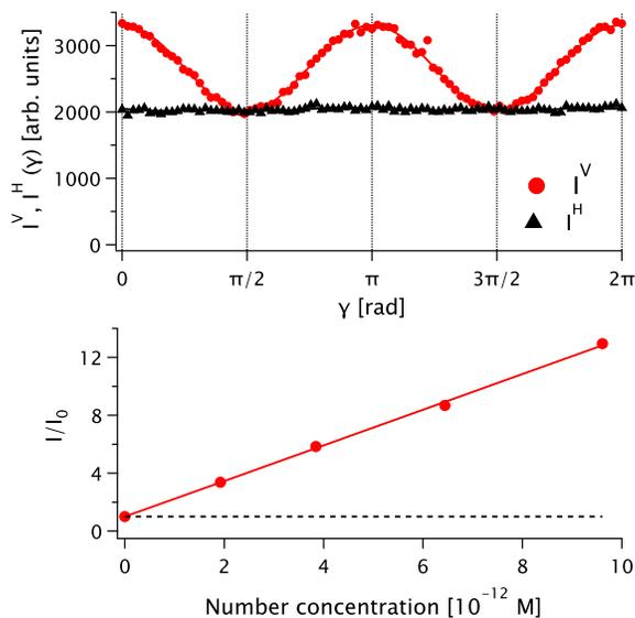
Figure 2: Sample NTP-1. Top: Polar graph of the (red) vertically and (black) horizontally polarized HRS intensity  $I_{\text{HRS}}^{\Gamma}(\gamma)$  as a function of the fundamental polarization angle (symbols) and fits (lines). Bottom: dilution law for the same sample. The signal  $I_{\text{HRS}}^V(\gamma = 0)$  is normalized to the solvent signal  $I_0$ . The slope of its dependence with respect to the particle concentration yields the first hyperpolarizability  $\beta$ .
