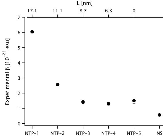
Figure 3: Left axis: first hyperpolarizability  $\beta$  for all the samples, identified on the bottom axis (solid black dots). Error bars are smaller than the symbol size. For NTPs, the arm length  $L$  is given on the top axis.
