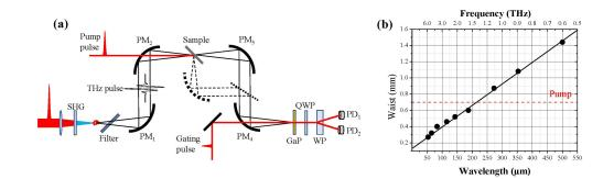
Fig. 1. Setup of the optical-pump THz-probe experiment. PM, parabolic off-axis mirror; QWP, quarter-wave plate; WP, Wollaston prism; PD: photodiode. b) Evolution of the waist size of the THz beam on the sample versus the wavelength or THz frequency. The black line is a linear fit of the waist size versus the THz frequencies. The dashed red line indicates the pump waist size seen by the different THz spectral components.
