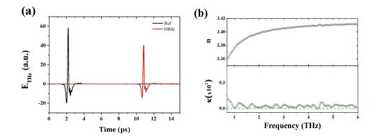
Fig. 2. a) In black the temporal evolution of the THz pulse generated in our setup. In red, temporal evolution of the THz pulse transmitted by the HRSi wafer. b) Evolution of the real part of the index of refraction n and extinction coefficient  $\kappa$  of the HRSi wafer in between 0.7 and 6 THz.
