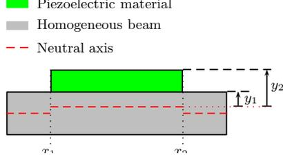
**Fig. 2** Positions of electrodes of the piezoelectric material with respect to the neutral axis ( $y_1$  and  $y_2$ ).
