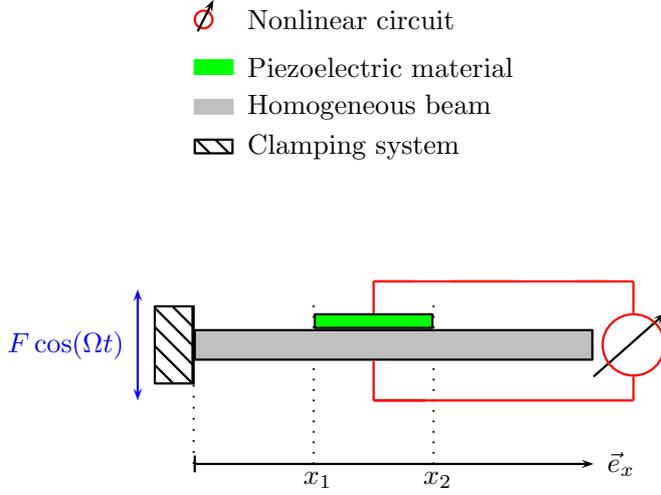
**Fig. 1** Scheme of the composite system: a homogeneous beam is patched with a piezoelectric material at  $x \in [x_1, x_2]$ . The piezoelectric material is coupled to a nonlinear circuit. The overall system is under lateral base excitation as  $F \cos(\Omega t)$ .
