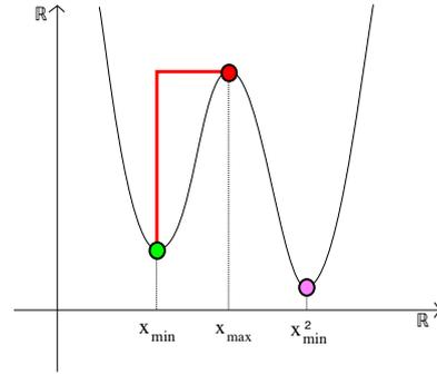
Fig. 4: Example of pairing by persistence: the abscissa  $\mathbf{x}_{\max}$  of the local maximum in red is paired by persistence relatively to  $f$  with the abscissa  $\mathbf{x}_{\min}$  of the local minimum in green, since its image by  $f$  is greater than the image by  $f$  of the abscissa  $\mathbf{x}_{\min}^2$  of the local minimum drawn in pink.
