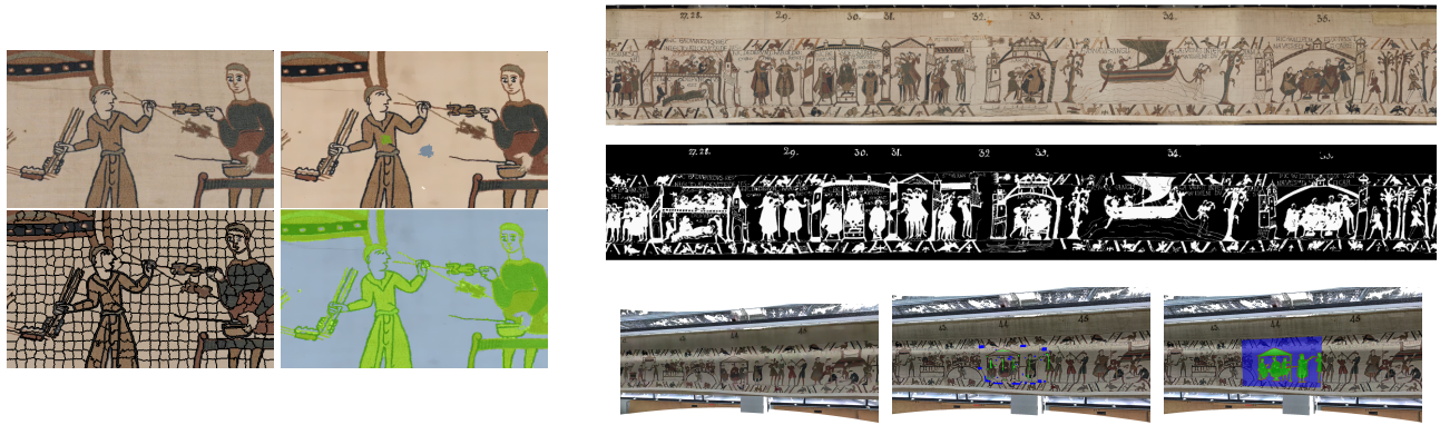
Figure 3. Semi-supervised segmentation of the Bayeux Tapestry. Left: superpixel-based segmentation of a single scene (initial image, image with seeds, image partition with supervertices using a regular grid of seeds, and segmentation result). Right, first and second rows: segmentation of the foreground on 2D images (initial image and segmentation result). Right, third row: 3D point cloud segmentation (from left to right: initial image, image with initial labels, segmentation result).
