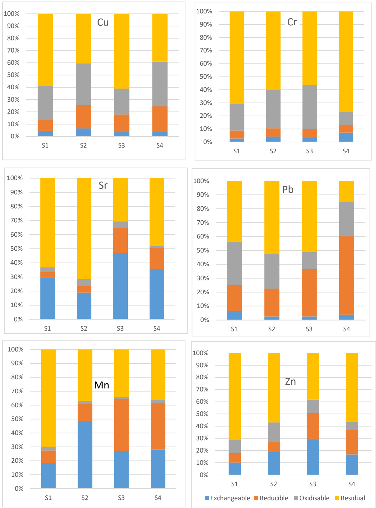
Fig. 2. Percentage distribution of metals between various fractions determined by the BCR extraction test in the soils from the four sampling sites.
