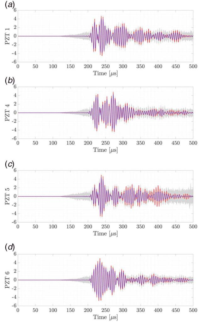
**Fig. 4** Monte Carlo prediction for GP-NARX healthy model of different paths, where —, mean of the GP-NARX metamodel; ···, experimental observation; ■,  $3\sigma$  uncertainty bounds: (a) path 2 → 1, (b) path 2 → 4, (c) path 2 → 5, and (d) path 2 → 6
