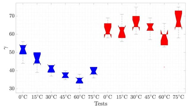
**Fig. 12** Box plot of the index  $\gamma$  (outliers) for healthy versus damaged assuming temperature changes to the PZT path 2–4. The reference model is identified using a virtual signal compressed by PC.
