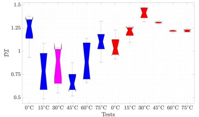
**Fig. 8** BoxPlot of the  $DI$  for ■ healthy versus ■ damaged assuming temperature changes for the PZT path 2–4. The reference model is identified using the temperature of 30 °C using the training data described by ■.
