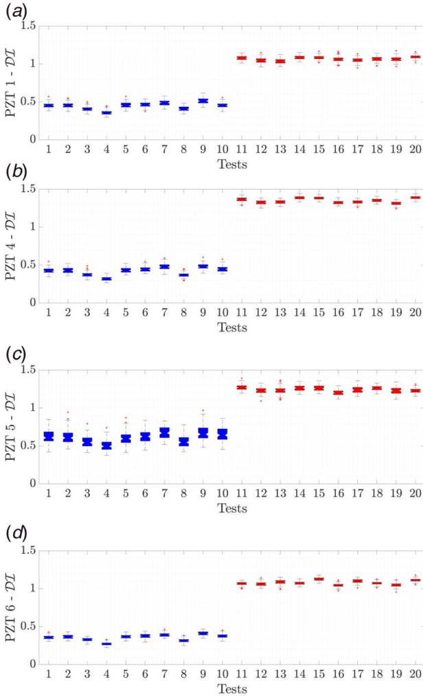
**Fig. 5** Box plot of the  $DI$  considering some paths by propagating uncertainties using Monte Carlo simulations with 100 runs: ■ healthy versus ■: (a) path 2 → 1, (b) path 2 → 4, (c) path 2 → 5, and (d) path 2 → 6
