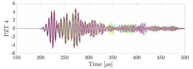
**Fig. 7** Temperature effect in one realization of healthy state signals: 0 °C, 15 °C, 30 °C, 45 °C, 60 °C, and 75 °C
