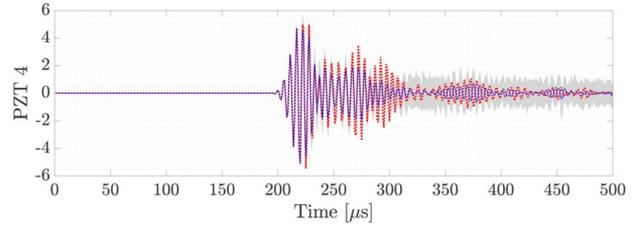
**Fig. 11** Monte Carlo prediction for GP-NARX model obtained by the virtual signal for healthy condition where – is mean of the GP-NARX metamodel, ... is experimental observation in a randomly temperature test, and ■ is  $3\sigma$  uncertainty bounds
