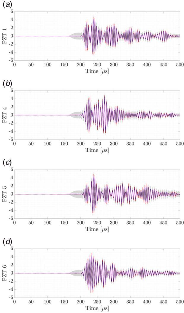
**Fig. 3** Model-predicted output for GP-NARX healthy model of different PZTs paths, where —, GP-NARX metamodel; ···, experimental observation; ■,  $3\sigma$  uncertainty bounds: (a) path 2 → 1 with fit of 85.7%, (b) path 2 → 4 with fit of 86.6%, (c) path 2 → 5 with fit of 82.2%, and (d) path 2 → 6 with fit of 88.2%
