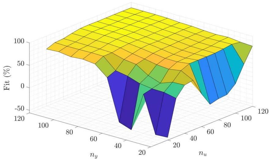
**Fig. 2** Order selection with focus in model-predicted output for the PZT path 2–4 at 30 °C
