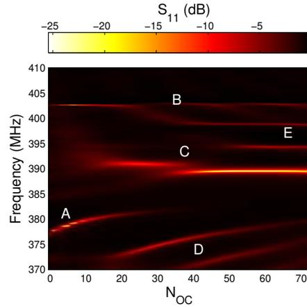
FIG. 5.  $S_{11}$  coefficient magnitude of the resonator (with the corrective capacitance) as a function of frequency and number of floating electrodes in each mirror  $N_{OC}$ . Port impedance is  $50 \Omega$ .
