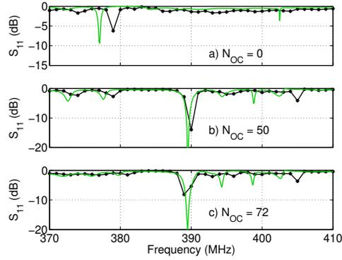
FIG. 4. Fit between the "slice model" (Green) and the full FEM simulation (Black) of the (a)  $N_{OC} = 0$ , (b)  $N_{OC} = 50$  and (c)  $N_{OC} = 72$  resonator by using a capacitance connected between each OC electrode and the ground.
