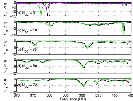
FIG. 6. Simulated (green) and measured (black)  $S_{11}$  magnitude spectra for resonators with  $N_{OC} = 0, 10, 30, 50$ , and  $72$ . Port Impedance is  $50 \Omega$ . For the  $N_{OC} = 0$  case, the complete resonator simulation is also shown (magenta).
