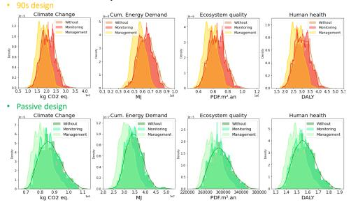
**Fig. 4.** Comparison of smart and conventional building alternatives, for the 90s design (graphs on the top) and the passive design (graphs on the bottom).
