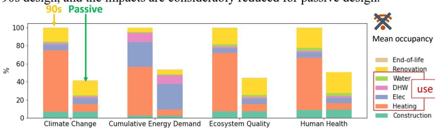
**Fig. 2.** Contribution analysis for the “without sensor” alternative and the mean occupancy.
