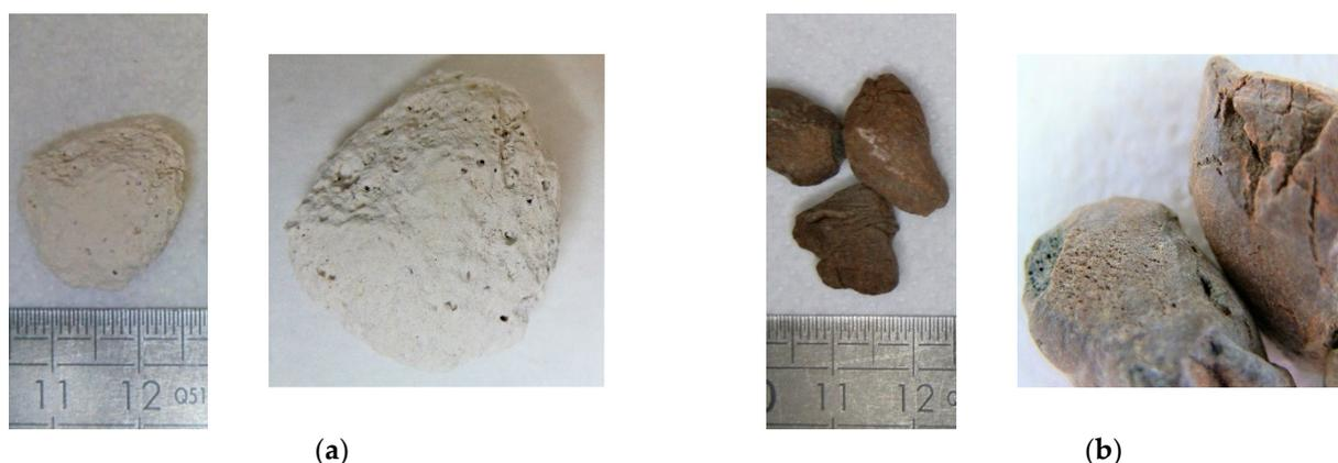
**Figure 1.** Materials used in this study; (a) cellular concrete waste; (b) expanded schist.
