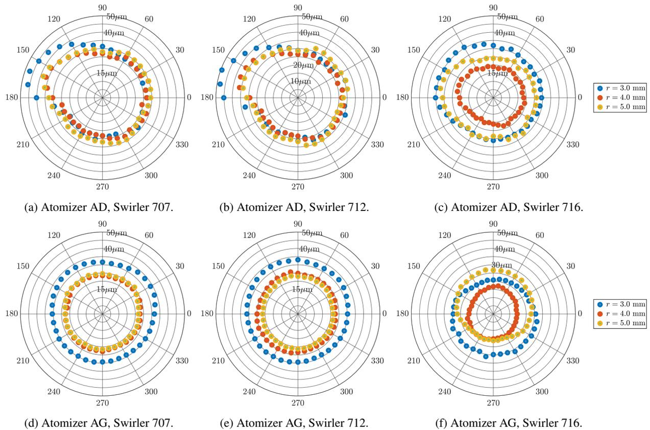
Fig. 3: Circumferential distribution of the Sauter mean droplet diameter  $d_{32}$ . For each data point the azimuthal angle on the graph corresponds to the azimuthal angle in the experiment, the color of the point to the radial coordinate of the measurement point, and the radial position in the graph corresponds to the value of  $d_{32}$  (the gray circles correspond to 5, 10, 15...  $\mu\text{m}$  as indicated in the graphs when this is possible). Measurements acquired at  $z = 2.5$  mm.
