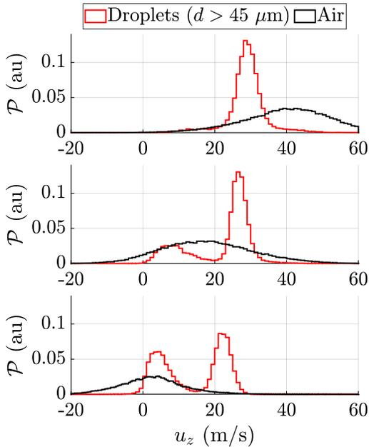
Fig. 8: In red, axial velocity histogram for large droplets (diameter greater than  $45 \mu\text{m}$ ) at 3 radial positions (from top to bottom,  $r = 4, 5$  and  $6$  mm, all taken at  $z = 5$  mm). In black, air axial velocity histogram from LDV measurements.
