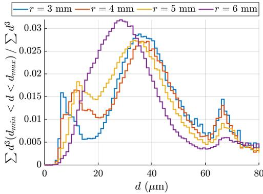
Fig. 6: Volumetric droplet size histograms measured at four radial positions  $z = 5$  mm above the backplane. The plots correspond to the fraction of the total liquid volume for each droplet diameter class in the histogram.
