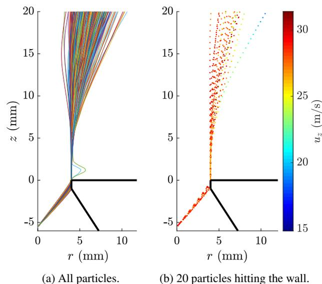
Fig. 15: Backward - forward lagrangian particle tracking of all droplets that pass inside the control volume (0.5 mm diameter torus around the point of interest at  $r = 4$  mm,  $z = 5$  mm). On the right, trajectories are colored by axial velocity.
