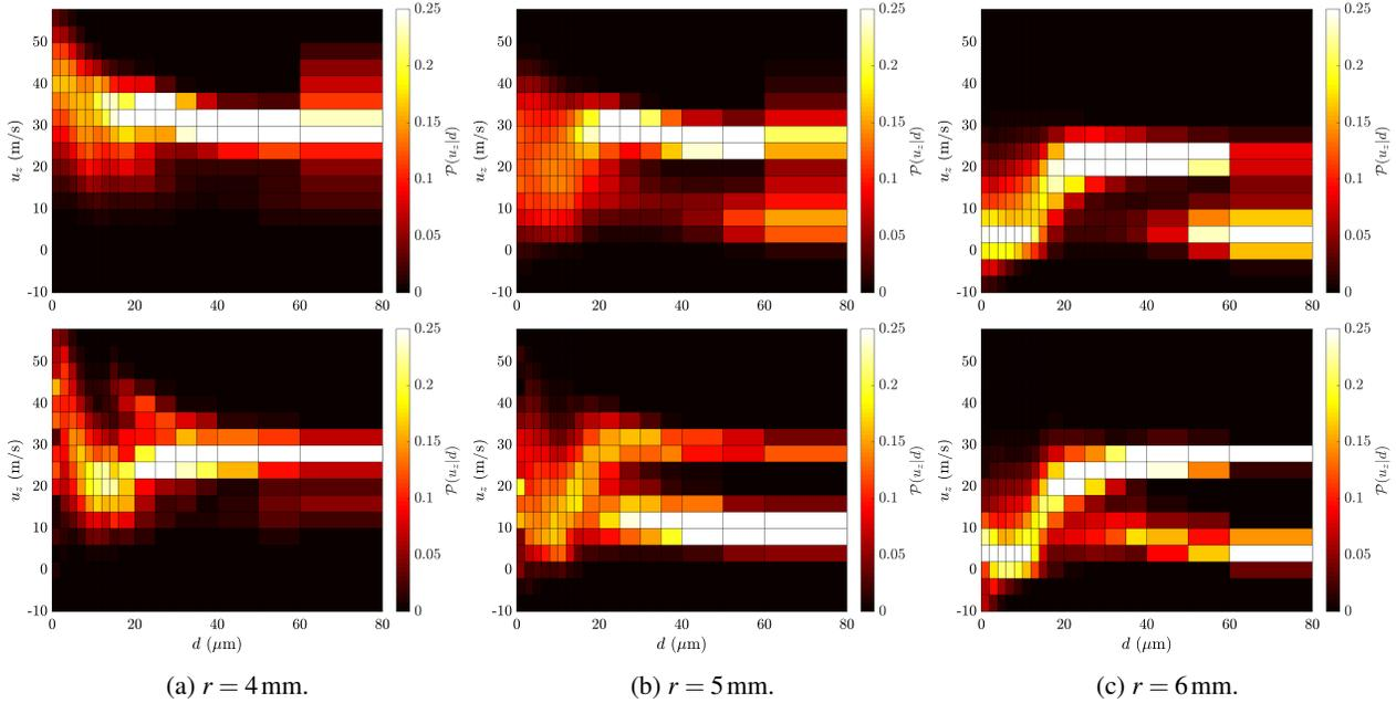
Fig. 7: Probability of axial velocity conditioned by the droplet diameter at  $z = 5$  mm and at radial positions  $r = 4, 5$  and  $6$  mm. On the top row, experimental results measured by PDA. On the bottom row, simulation (LES) results that will be discussed in the LES section. In both cases, circumferential averaging is performed.
