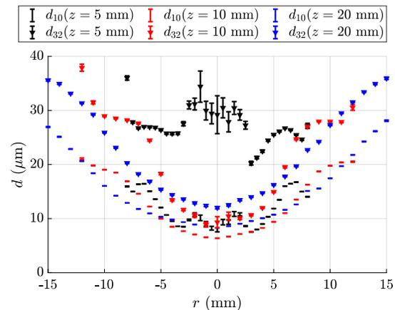
Fig. 4: Radial profiles of mean droplet diameter  $d_{10}$  and Sauter mean diameter  $d_{32}$  obtained at  $z = 5, 10$  and  $20$  mm above the backplane (red dotted lines in Fig. 5). Swirler 707. Error bars indicate the 95% statistical confidence interval obtained from bootstrapping.
