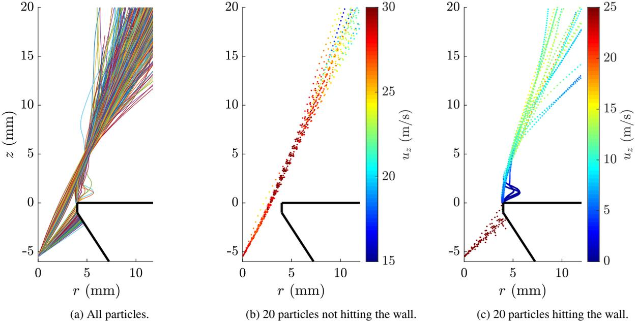
Fig. 14: Backward - forward Lagrangian particle tracking of all droplets that pass inside the control volume ( $0.5$  mm diameter torus around the point of interest at  $r = 5$  mm,  $z = 5$  mm). In black, geometry of the upper part of the injector. On the right, trajectories are colored by axial velocity.
