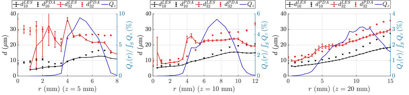
Fig. 13: Comparison of mean (black) and Sauter mean (red) diameters from the LES with PDA measurements. Three measurement sections are considered ( $z = 5, 10$  and  $20$  mm). Azimuthal averages are performed in both cases. On the right axis, the radial distribution of the axial liquid volume flux is shown as a blue solid line.
