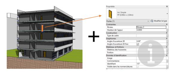
**BIM** (Building Information Model) = 3D objects with properties (type, quantities, etc.) representing a building site
