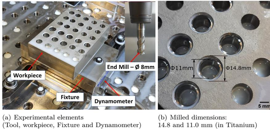
Figure 3: Experimental setup
