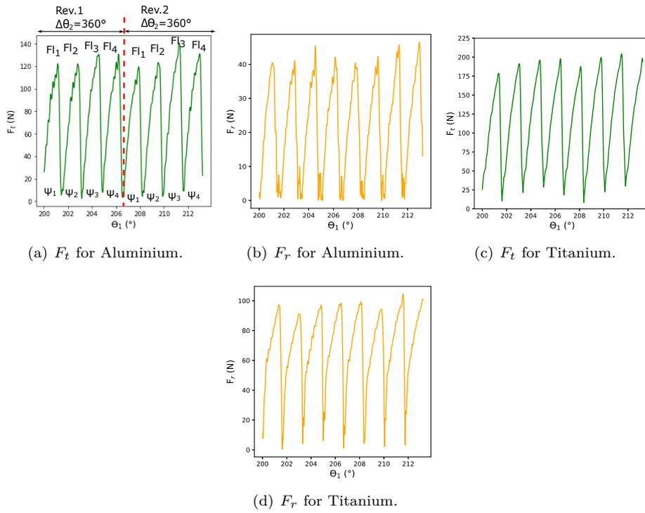
Figure 7: Calculated  $F_t$  and  $F_r$  during 2 revolutions in circular milling of Aluminium and Titanium (window on  $\theta_1 = [200^\circ - 213^\circ]$ ) at  $f_z = 0.1$  mm/th and  $V_c = 40$  m/min
