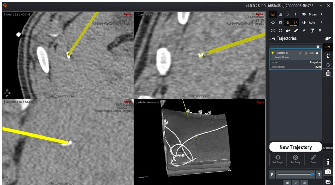
Figure 4. Screenshot of the planning software (home-made software). The needle trajectory (in yellow) is planned by defining the entry (skin) and the target points.
