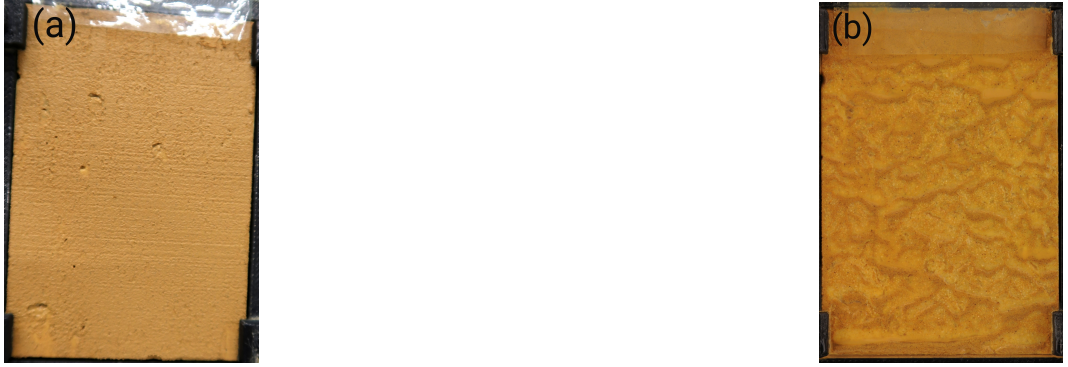
Fig. 2: (a) Initial state and (b) final pattern for \alpha = 85^\circ and \Delta T = 3.3 K (image size: 80 \times 55 mm).
