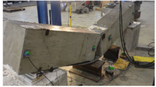
Figure 13. Experimental failure of SP1-2 beam.
