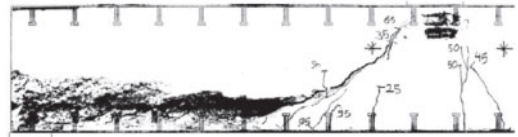
Figure 9. Experimental final crack pattern for SP1-1 beam.
