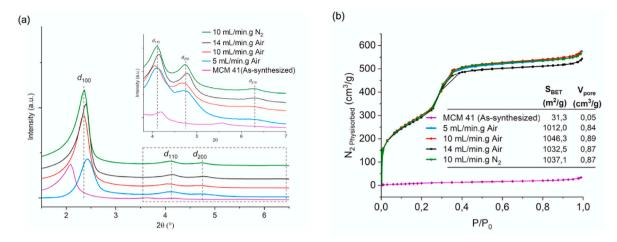
Fig. 2. X-ray diffractograms (a) and N<sub>2</sub> physisorption isotherms at -196 °C (b) of MCM-41 before and after calcination under air and N<sub>2</sub> atmosphere.
