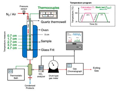
Fig. 1. Experimental setup employed for the thermal detemplation.
