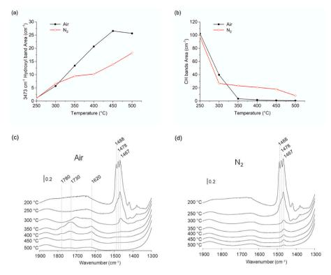
**Fig. 6.** Evolution of hydroxyl (a) and CH (b) stretching bands as a function of the temperature with and without oxygen. IR spectra, in 1300–1900 cm<sup>-1</sup> region at different temperatures in the presence (c) and absence (d) of oxygen.
