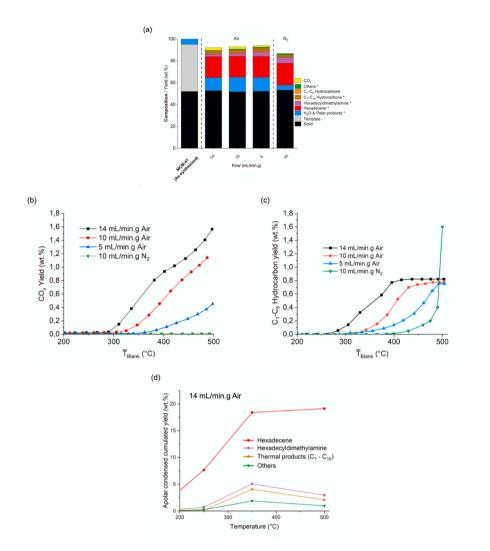
**Fig. 4.** Products yield under different flows of air and  $N_2$ . (a). The yield of (CO<sub>x</sub>) CO and CO<sub>2</sub> (b) and  $C_{1-}C_6$  hydrocarbons (c) as a function of the average temperature of the sample bed without CTA<sup>+</sup>. Cumulative: condensed products yield as a function of the input temperature under 14 mL/min.g Air (d).
