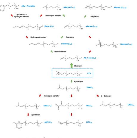
Fig. 5. Reaction scheme of MCM-41 detemplation with and without oxygen. <u>Notation</u>: Hexadecyltrimethylammonium (CTA<sup>+</sup>), Hexadecene (Alk-1-ene), Hexadecyldimethylamine (DMAC<sub>16</sub>), Olefin-amines (not-detected\*, DMAC = 16), Alkyl-Pyridines (AKPYC<sub>16</sub>), Hexadecylformamide (FMAC<sub>16</sub>), Hexadecanenitrile (NITC<sub>16</sub>), Pentadecylamine (DMAC<sub>15</sub>).
