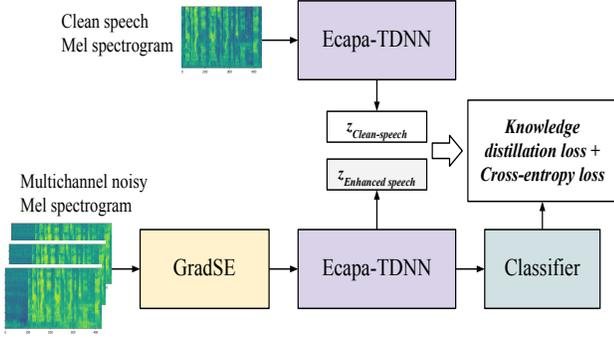
**Fig. 2.** Joint optimization of multichannel speech enhancement with SV using KD loss. Embedding generated by ECAPA-TDNN for clean speech Mel spectrogram is considered as the teacher network. Embedding generated by joint optimized network on multichannel noisy Mel spectrogram is considered as the student network.
