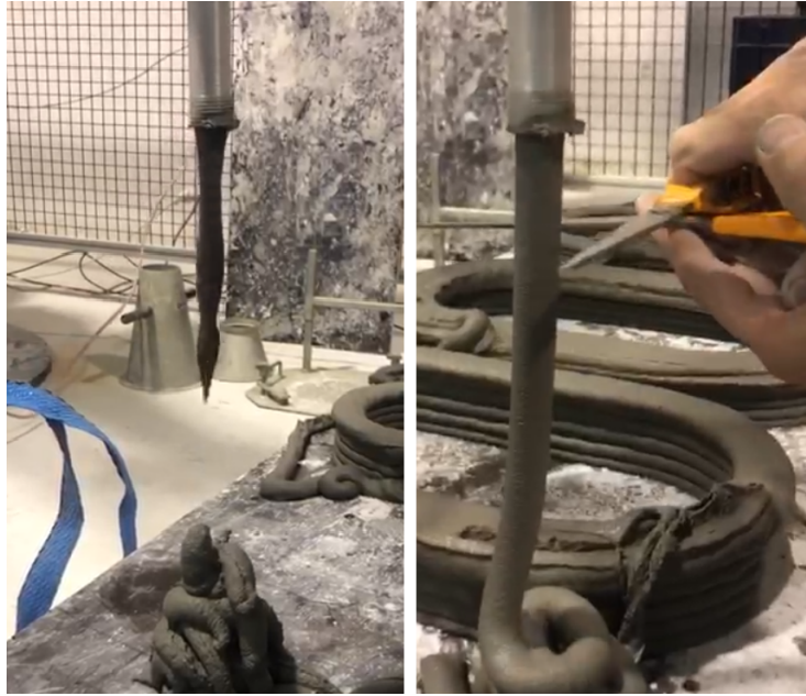
Figure 9: Lace behavior without (left) and with 0,2% fiber by volume (right) - same cement formulation.
