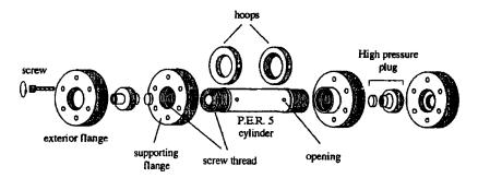
FIGURE 1 View of the parts of the disassembled high pressure cell. The hoops have been moved upwards for clarity in the drawing.
