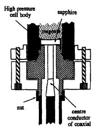
FIGURE 3 Coupling of microwaves in the pressure vessel through a coaxial line.
