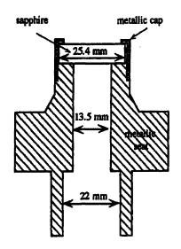
FIGURE 2 A two-dimensional view of the high pressure plug.
